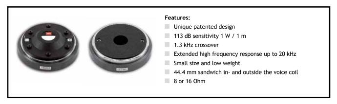
BMS 4544 is a powerful 1" professional compression driver that delivers excellent sonic quality in a small package. The BMS exclusive voice coil technology employs light weight Cooper clad Aluminum wire wound inside and outside of the Kapton $^{\text{TM}}$  former to improve the heat dissipation.
