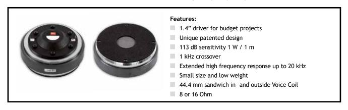
BMS 4554 is a powerful 1.4" professional compression driver that delivers outstanding sonic quality in a small package. The BMS exclusive voice coil technology employs a light weight Copper clad Aluminum wire wound inside and outside of the Kapton $^{\rm m}$  former to improve the heat dissipation, dramatically increasing the acoustic output and reliability of the driver while minimizing the power compression.
