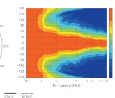
\* Horn measured using LAVOCE DN10.17T compression driver All specifications subject to change without notice\_B.a
